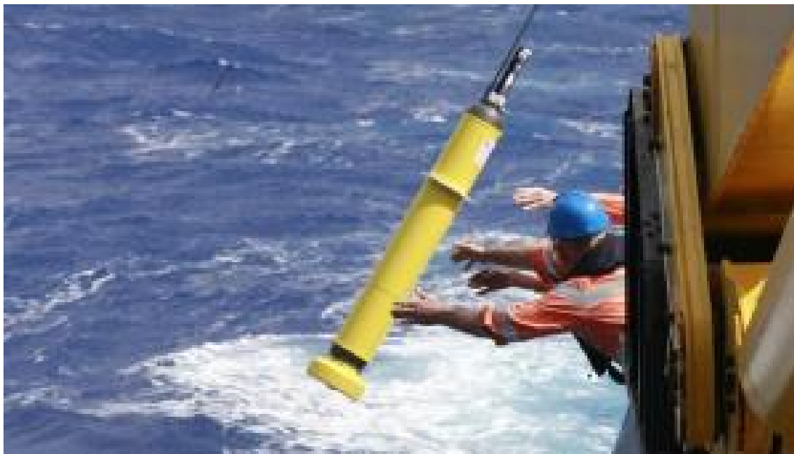
An Argo robotic profiling instrument being deployed from the research vessel, Southern Surveyor. (Credit: Alicia Navidad)
